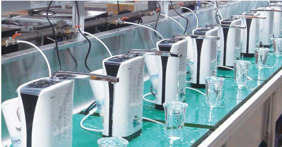
100% testing and inspection system to check for normal operation and water leakage
